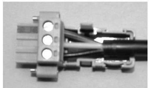
**Step 2:** Insert your pre-wired connector (with the screws facing up) into the bottom shell. (See manual for cable wiring instructions).
