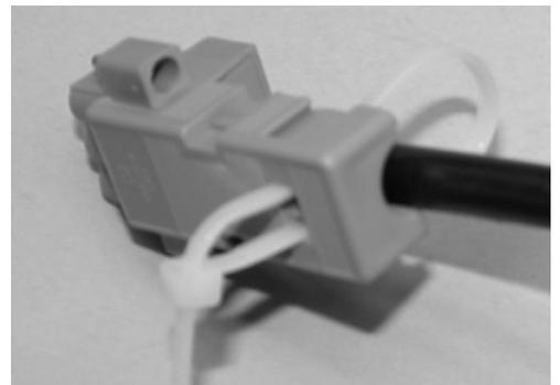
**Step 3:** Insert the wire tie from the bottom shell, loop around the cable and come back out of the opposite hole in the bottom shell.
